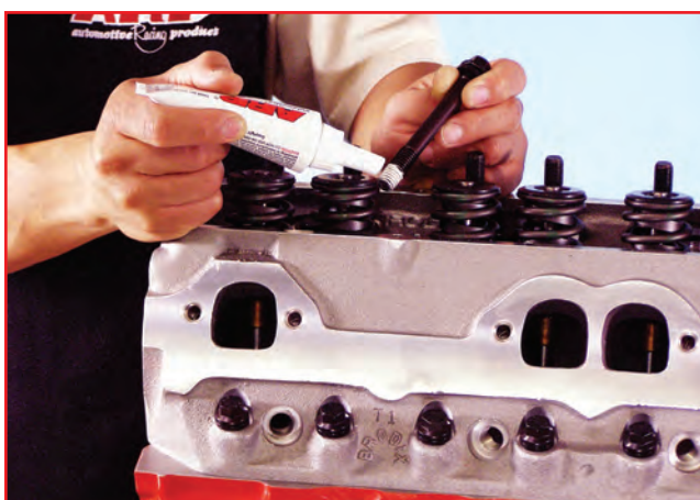
4. Seal all threads extending into a water jacket with ARP thread sealer. Lubricate all threads on dry deck and/or main cap applications with ARP Ultra-Torque fastener assembly lubricant.
