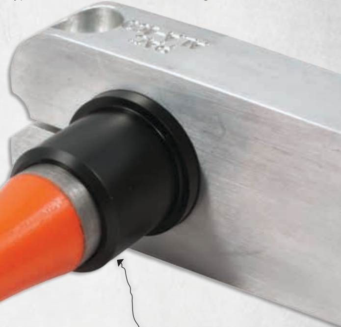
Bushing installed on sway bar
