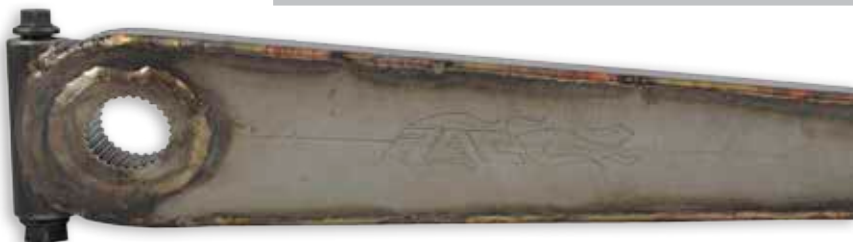
PAC-300343 cut to fit the spline clamp tube
