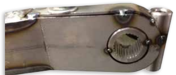
Pro Fabricator Link Arm tacked together
