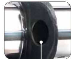
LIGHTENING HOLES IN ALL ROD THROWS (EXCEPT 3.480 STROKE)
