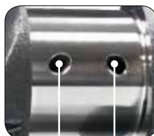
STRAIGHT SHOT & CHAMFERED OIL HOLES
