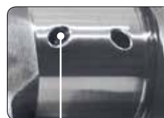
STRAIGHT SHOT & CHAMFERED OIL HOLES
