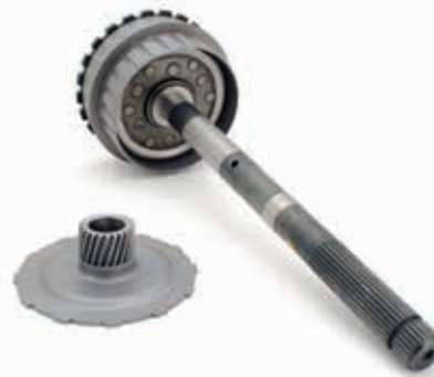
#747500 1.82 Standard Length w/ Reinforced Carrier
