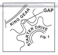
Measure the "gap" (Clearance) between the starter Drive Gear and Ring Gear. This should not be less than .025" (0.63mm) and not more than .060" (1.52mm). A paper clip is approx .035" (0.88mm) and may be used as a gauge.
